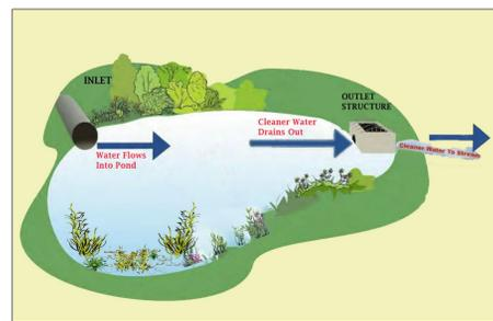
Figure 2: Function of stormwater ponds in removing nutrients from urban stormwater runoff. Processes such as nutrient uptake by vegetation, microbial activity, and sediment trapping can enhance nutrient removal rates to improve downstream water quality.
