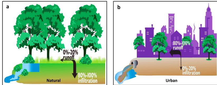
Figure 1: (a) In natural environments, the majority of stormwater infiltrates into the groundwater, while (b) in urban areas, the majority of stormwater runs over impervious surfaces into nearby waterbodies creating downstream flooding and concerns of water quality.
