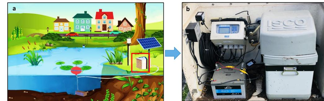
Figure 4: (a) Storm event sampling using a rain gauge, GatorByte sensor, and the autosampler powered by a solar panel to collect water samples as stormwater enters the pond and (b) an autosampler with the GatorByte sensor enclosed in a box.
