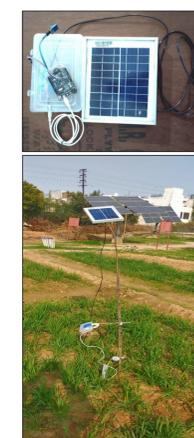
Fig 6. Developed IoT-based sensor system installed in field
