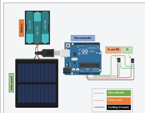
Fig 5. Schematic diagram IoT-based sensor system
