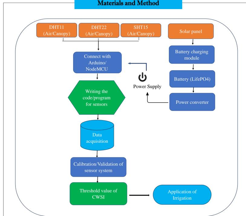
Fig 2. Methodological flowchart for application of sensor-based irrigation
