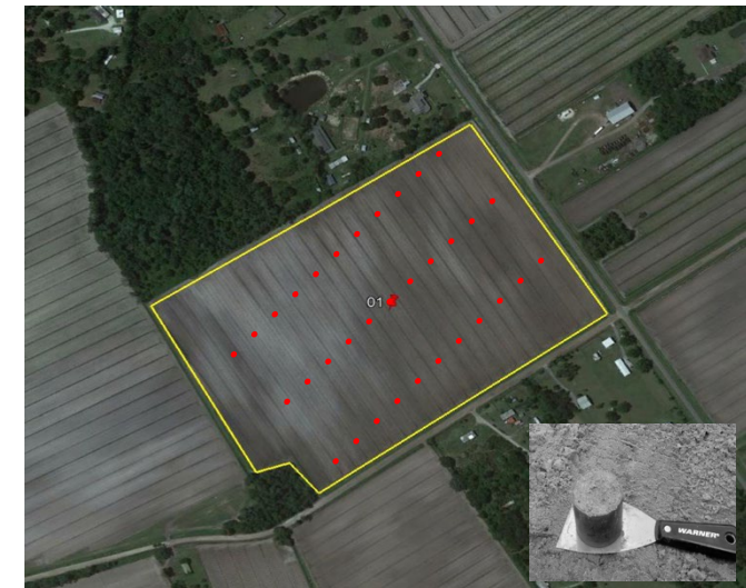
Fig.4. Soil undisturbed sampling in the selected sites on the layers 0-0.20 m and 0.20-0.40 m.
