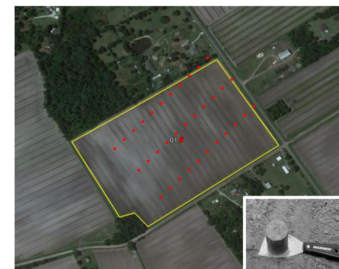
Fig.4. Undisturbed soil core sample from the selected sites sampled in the 0-0.20 and 0.20-0.40 m soil depth layers.
