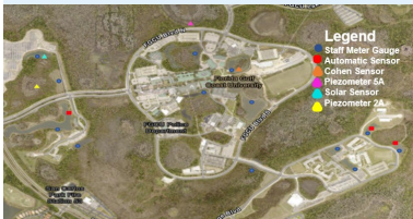
Figure 1: The FGCU campus. Buildings and paved surfaces show clearly against undeveloped areas, nearly all seasonal wetlands. Darkest features (open water) are stormwater ponds. Squares highlight two surface water sensors and two groundwater sensors that are used in this research. Stars show all other 17 surface water gauges and sensors.
