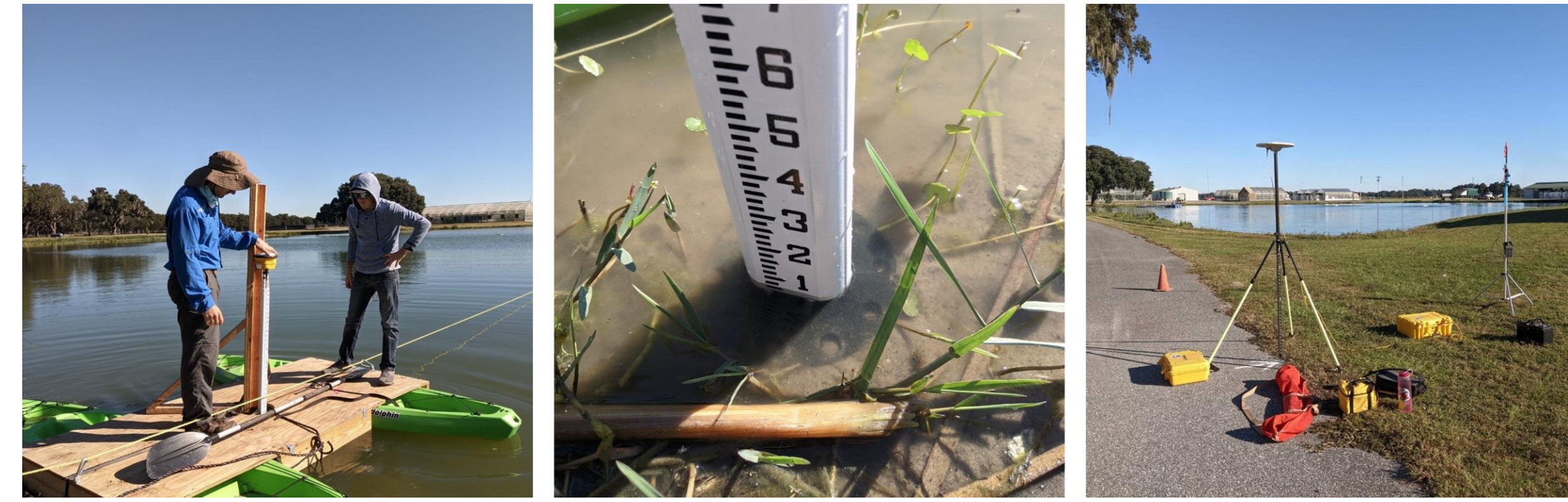
A stable barge suspended across the retention pond allowed for equal point distribution (left). A custom 3d printed topo-boot prevents the level pole from penetrating the silt during observation (center). GNSS base station (right).
