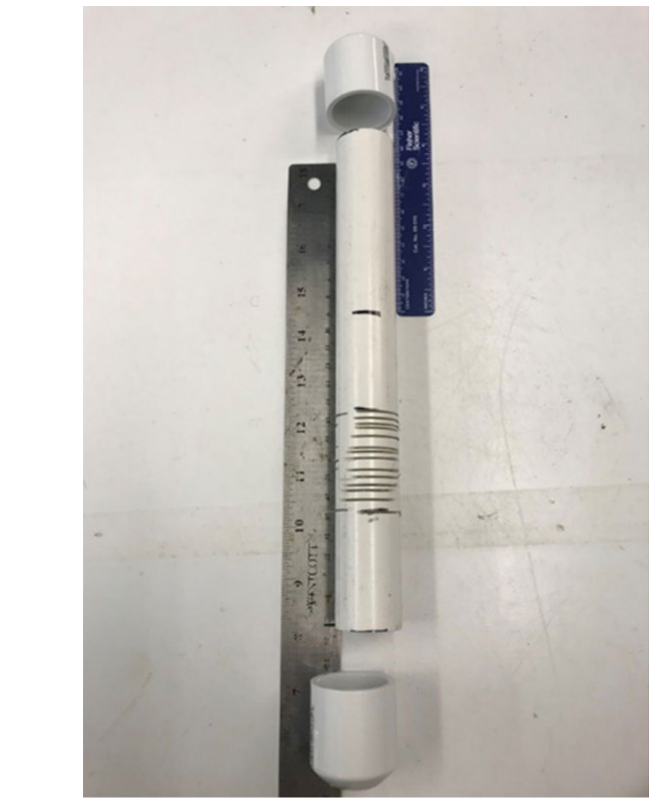
Figure 6: Schematic of porewater well & sipper design: 25cm long, 2.5" diameter PVC. Wells were placed 10cm in soil, slits were made between 5-10cm below the initial above ground section to collect at root zone. Wells were purged immediately prior to sampling.
