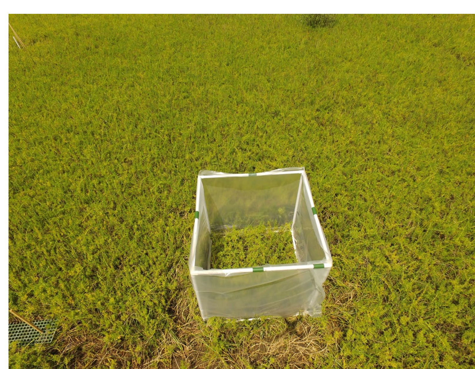
Figure 5: Warming chamber experimental design: 1.5m³ PVC chamber covered with 6 mil (152-µm) plastic film (Green-tek, Bladwin, Georgia, USA) to simulate average 2°C warming effect. Film allows 90% PAR thus trapping infrared radiation. (Chapman et al. 2018)
