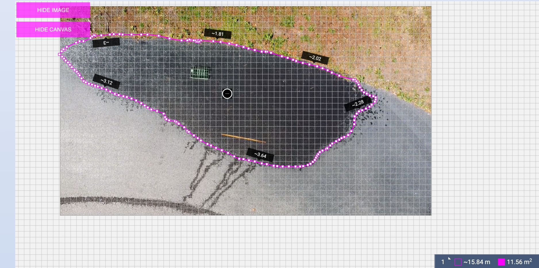
Example of using SketchAndCalc software to determine overspray area from image obtained by the drone.
