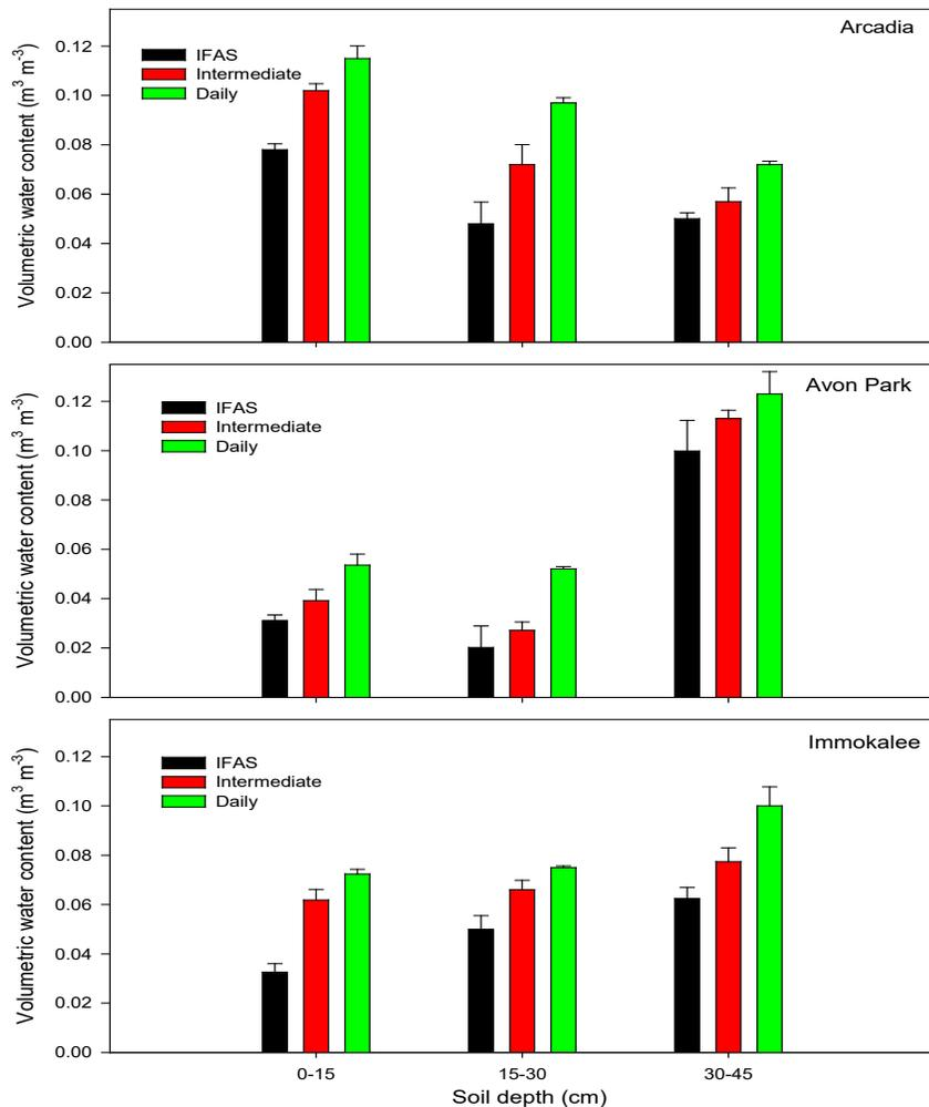
Keeping water in the top 0-30 cm improved water use for HLB affected trees. Greater moisture content beyond the root zone (at 45 cm) in Immokalee (bottom) could be due to capillary rise since the soils have a high water table and in Avon Park (middle) could be due to deep percolation because those soils are well drained.
