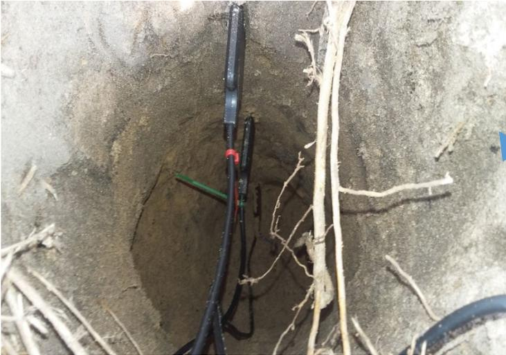
Water monitoring at grove scale and soil moisture measurement at 15, 30 and 60 cm soil depth
