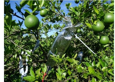
Use of sapflow sensors supported by a datalogger, solar panel, and 12-V battery (right and top)
