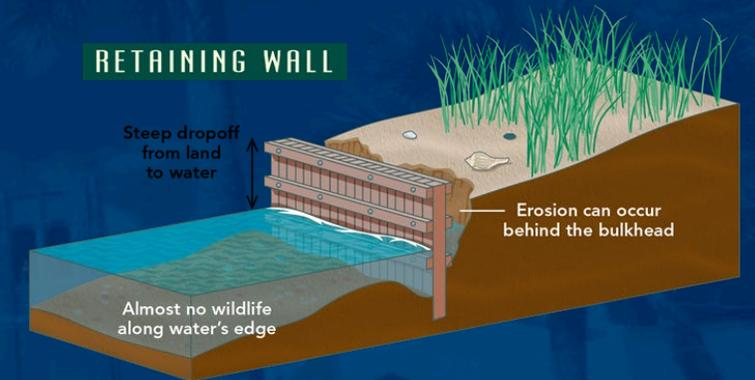
'Hard' infrastructure like retaining walls abruptly severs the ecological connection between the coast and water.
