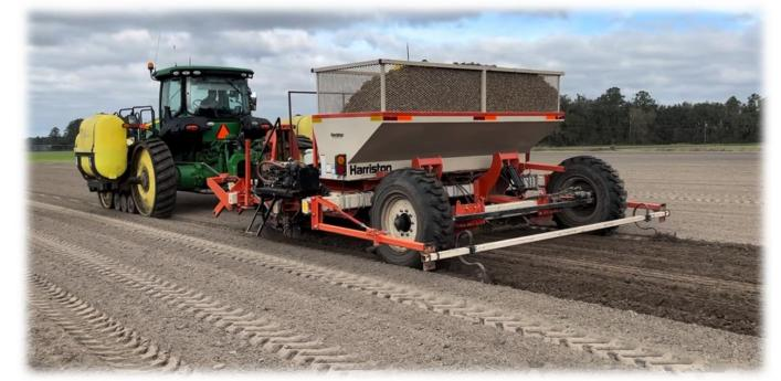
Figure 3. Potato planting using Six row potato planter during Spring-2023
