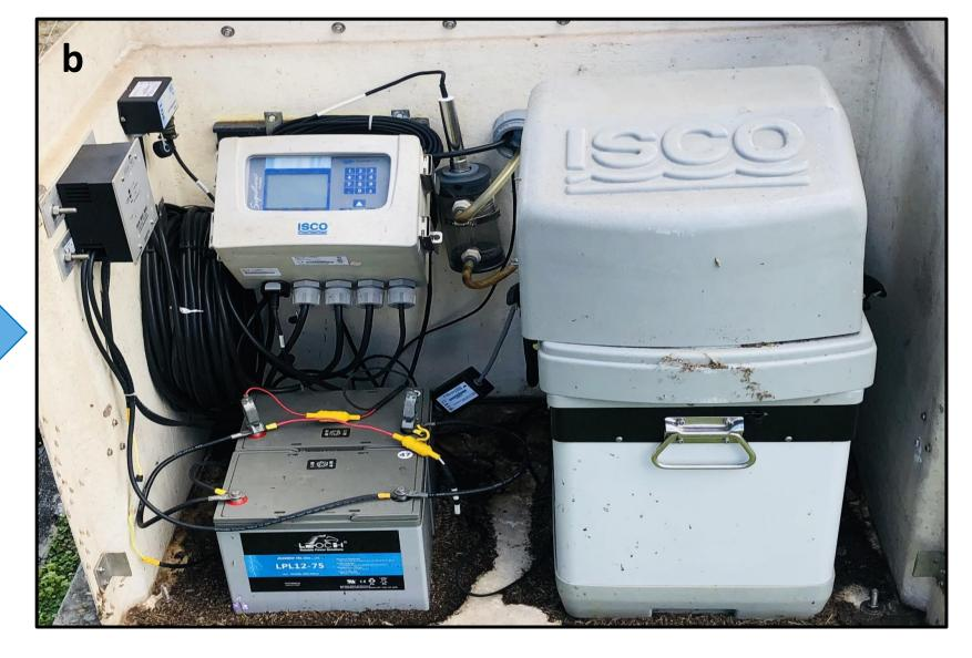
Figure 4: (a) Storm event sampling using a rain gauge, GatorByte sensor, and the autosampler powered by a solar panel to collect water samples as stormwater enters the pond and (b) an autosampler with the GatorByte sensor enclosed in a box.
