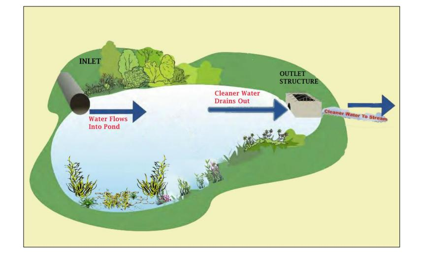
Figure 2: Function of stormwater ponds in removing nutrients from urban stormwater runoff. Processes such as nutrient uptake by vegetation, microbial activity, and sediment trapping can enhance nutrient removal rates to improve downstream water quality.
