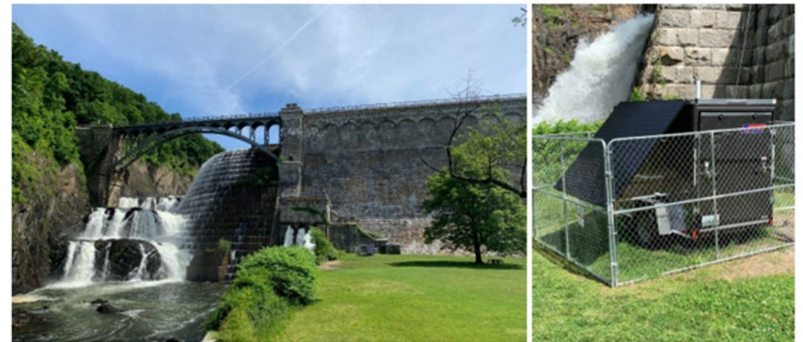
Solar-powered SATT system deployed at New Croton Dam, Croton River, NY
