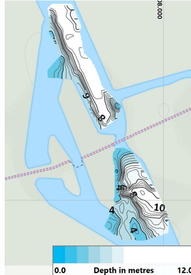
Bathy-Drone data interpolated on Reefmaster software
