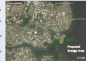
**Dredging:** Due to access issues in addressing the dredge scope, it is suggested to temporarily improve the existing dock for construction work, utilize a Kori Built marsh buggy fitted with excavator to allow for access to the Guachinanga Channel for woody vegetation and sediment removal and the use of Flexifloat interlocking modular barges that provide the ability to create floating barges that can be transferred to land for removal of dredge sediment.
