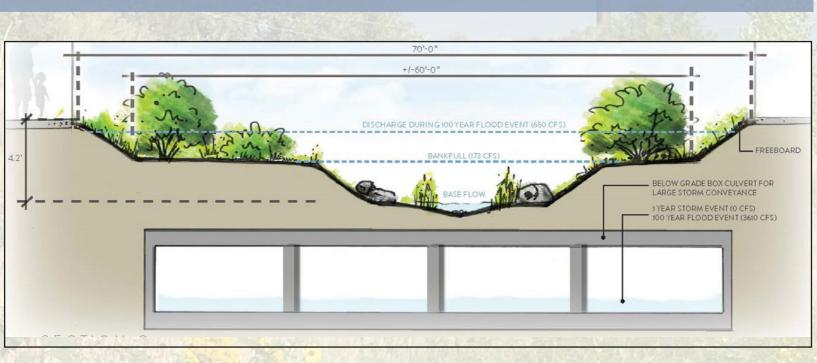
stormwater box culverts manages high-water flows during large storm events and moves the water below the road and railroad crossings allowing increased conveyance and removing the homes and businesses from the floodplain.
