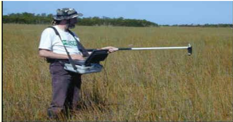
Figure 3. A library of South Florida land cover spectra is being built using handheld and laboratory spectroscopy.
