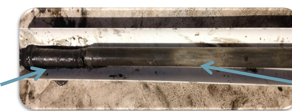
Fig. 5 Example of deep cores for examining "pre-muck" vs. "post-muck" assemblages.
