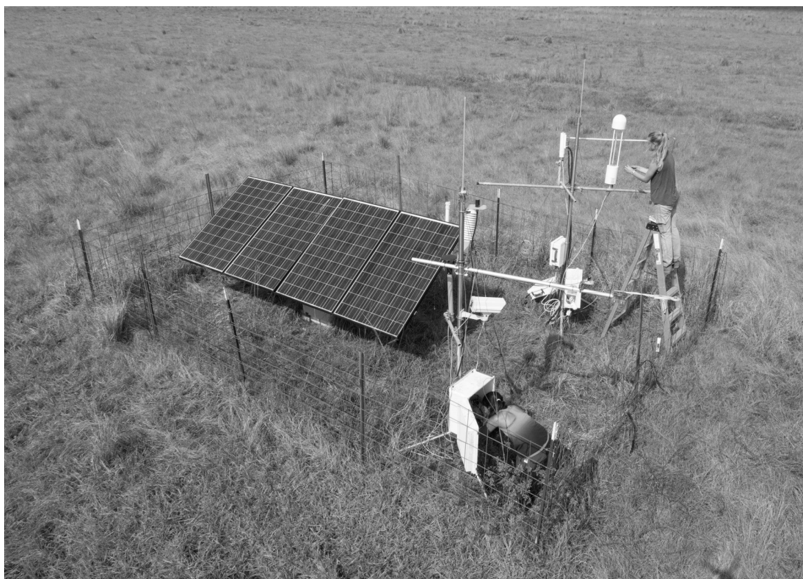
Buck Island Ranch staff make adjustments to an eddy covariance tower that measures carbon uptake and emissions from the grassland. Photo by Carlton Ward, Jr.
