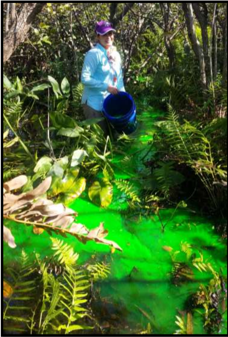
Large scale dye trial to visualize how water exits a tree island (December 2016)
