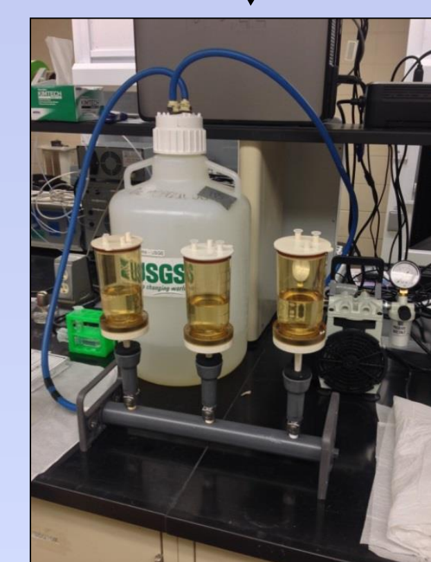
Filter water to concentrate eDNA
