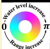
**Interferograms:** Detailed maps of phase changes occurring between the two acquisition dates. Each fringe cycle (blue-to-blue, yellow-to-yellow, etc.) represents 4 cm of water level changes.
