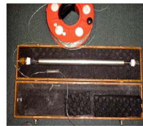
Thief or Kemmerer Sampler for collecting a sample at a particular depth
