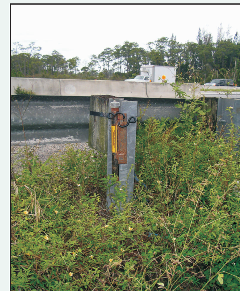
Figure 4. Barometric-pressure sensor deployed at WS_19 Imperial River.
