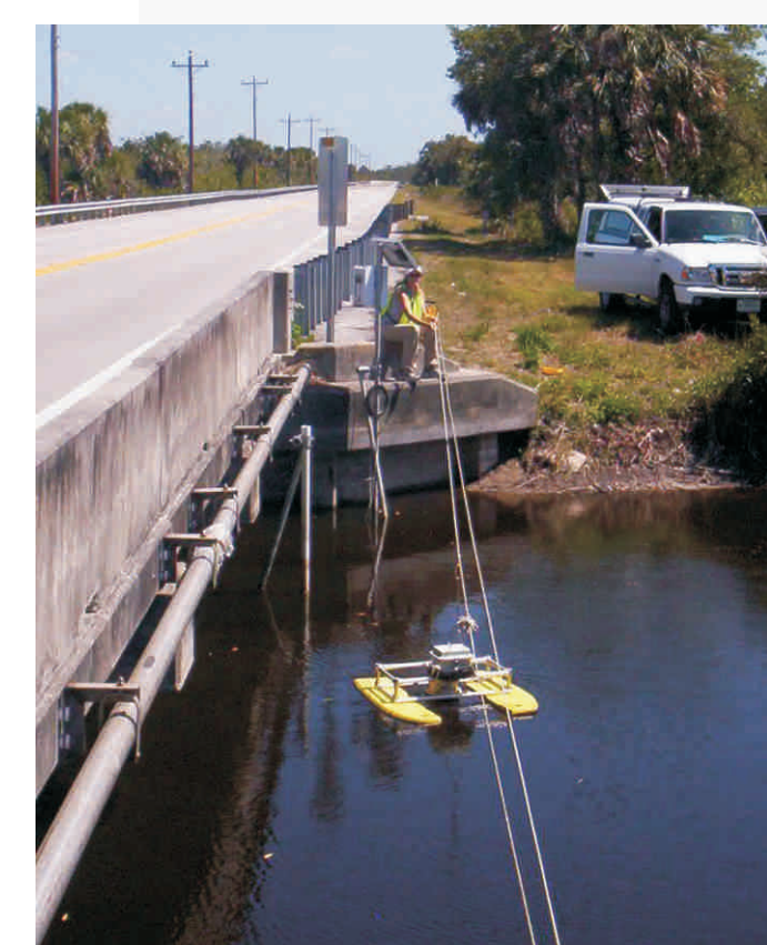
Clockwise from top: Performing an ADCP measurement at a station on Tamiami Trail; ADCP mounted to "boogie cat" used to measure bridges and river sites in the Ten Thousand Islands; Performing ADCP measurements thru a 13 hr tide cycle; SonTek SW on a mount for measuring discharge at culverts
