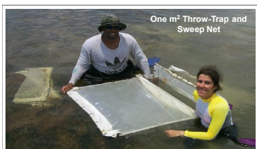
Figure 2. One-m 2 throw-trap and sweep net being used in Biscayne Bay. The cover net is in place with a sweep net in the throw-trap ready for use.
