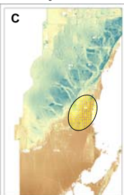
Figure C (bottom): the surface elevation in Miami-Dade as derived from a LIDAR survey. The East Glades (circled) are located in the coastal plain under the coastal ridge.
