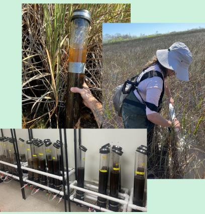
Soil core collection (top), experimental set-up in the lab (bottom).
