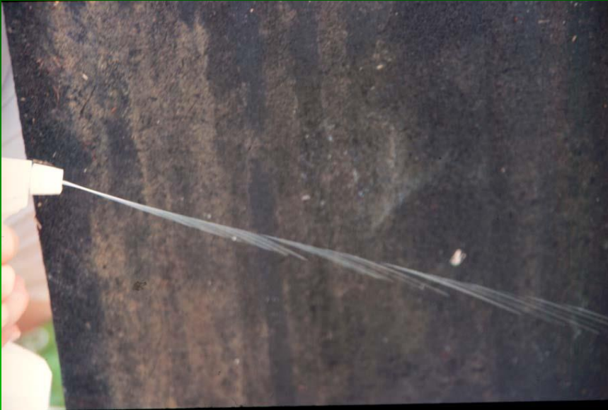
Poor Spray Pattern
