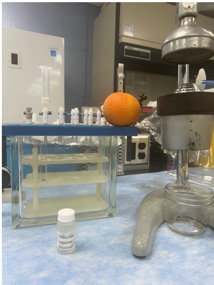
Isolation of LARL via C18 SPE, Buffer at pH = 6.7
