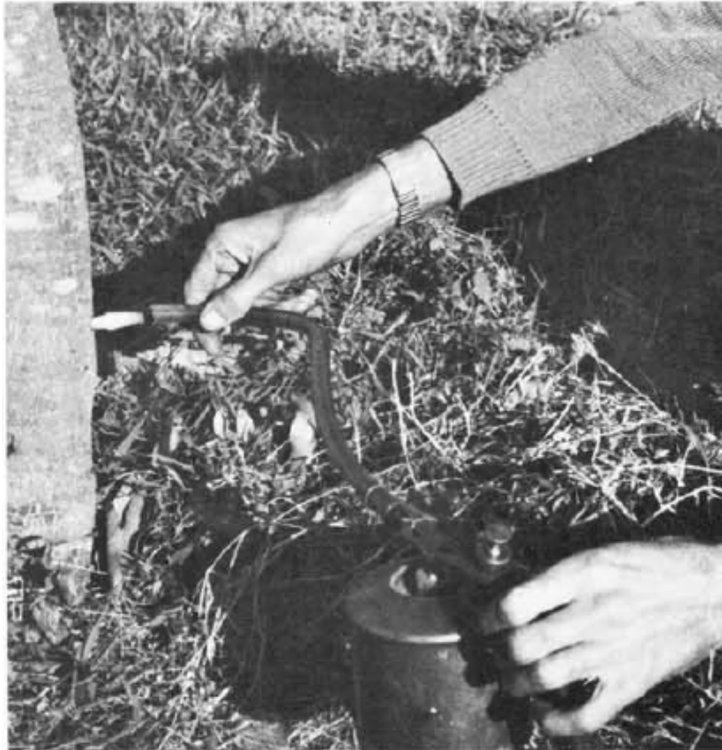
Fig. 1. Modified blowlamp injector.
