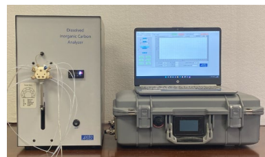
Apollo SciTech AS-c5 Dissolved inorganic carbon (DIC) analyzer
