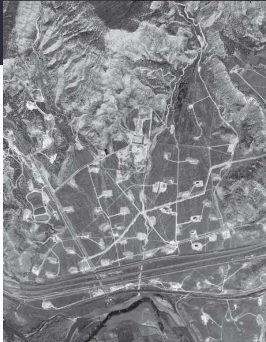
Model of oil and gas drill pads and resource roads overlying National Aerial Imagery Program (NAIP) imagery, near Rifle, Colorado, 2007 (USGS sir20105064 2010)
