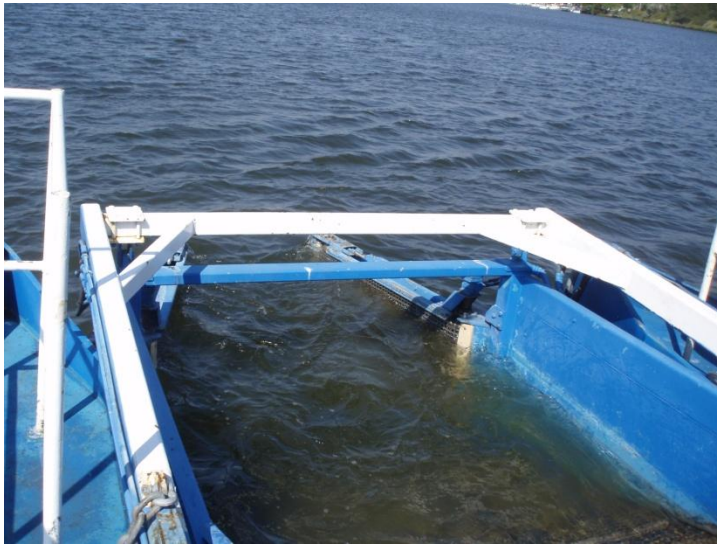
Intake conveyor ramp
