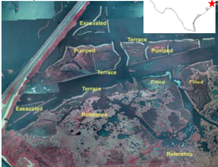
Figure 1: Study site in the Lower Neches Wildlife Management Area in Texas, USA. A reference area and three restoration construction methods with surrounding containment terraces are denoted.
