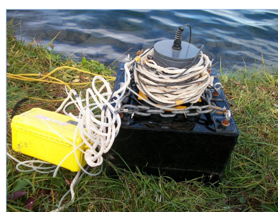
Figure 1: A dark benthic chamber before deployment. Grey cylinder houses a motor that powers an internal 1 rpm stir bar. Samples were collected at the surface via Tygon tubing.
