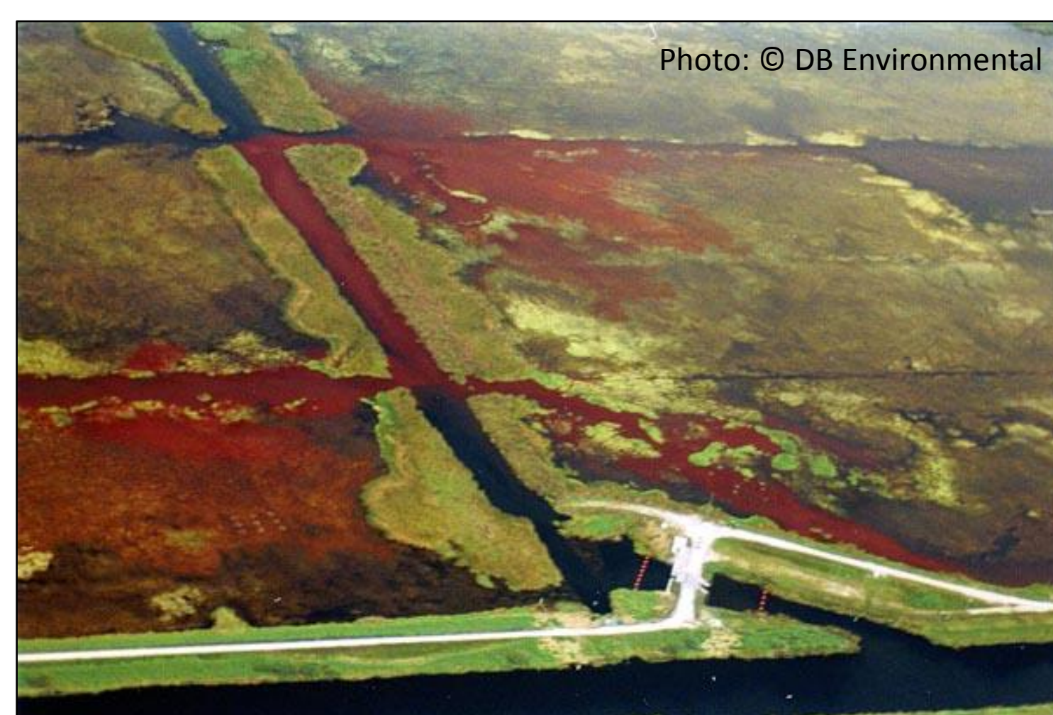
Fig. 2. Movement of the tracer Rhodamine-WT along short-circuit flow paths in a wetland.
