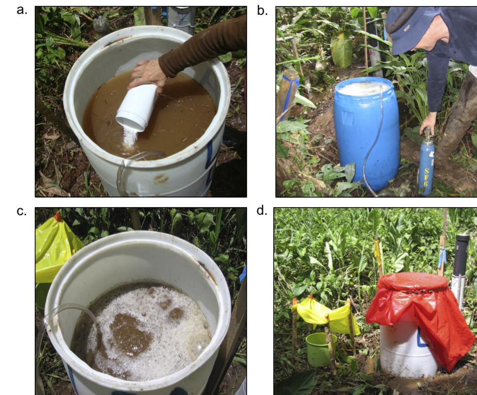
Fig. 5. Methods used in tracer preparation: (a) dissolving KBr into injection barrel filled with wetland water; (b) SF 6 canister connected via tygon tubing to a porous soaker hose in the bottom of the barrel; (c) dense stream of bubbles from SF 6 sparging; (d) reference bucket tented with plastic to prevent direct rainfall and minimize evaporation (left) and injection barrel covered with plastic to prevent SF 6 volatilization prior to tracer release (right).
