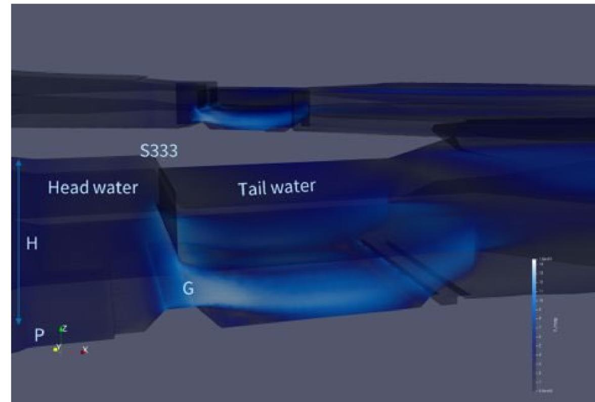
S333 gated structure design. Spillway with a lift-gate resting on it 3 ft from canal floor
