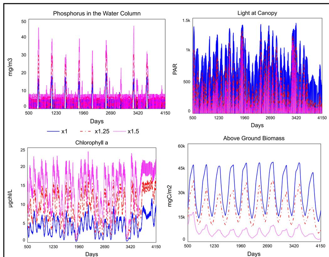
Figure 4: Simulations run for increased phosphorus in the water column and the projected impacts on light, chlorophyll concentration, and *Thalassia testudinum* above ground biomass.
