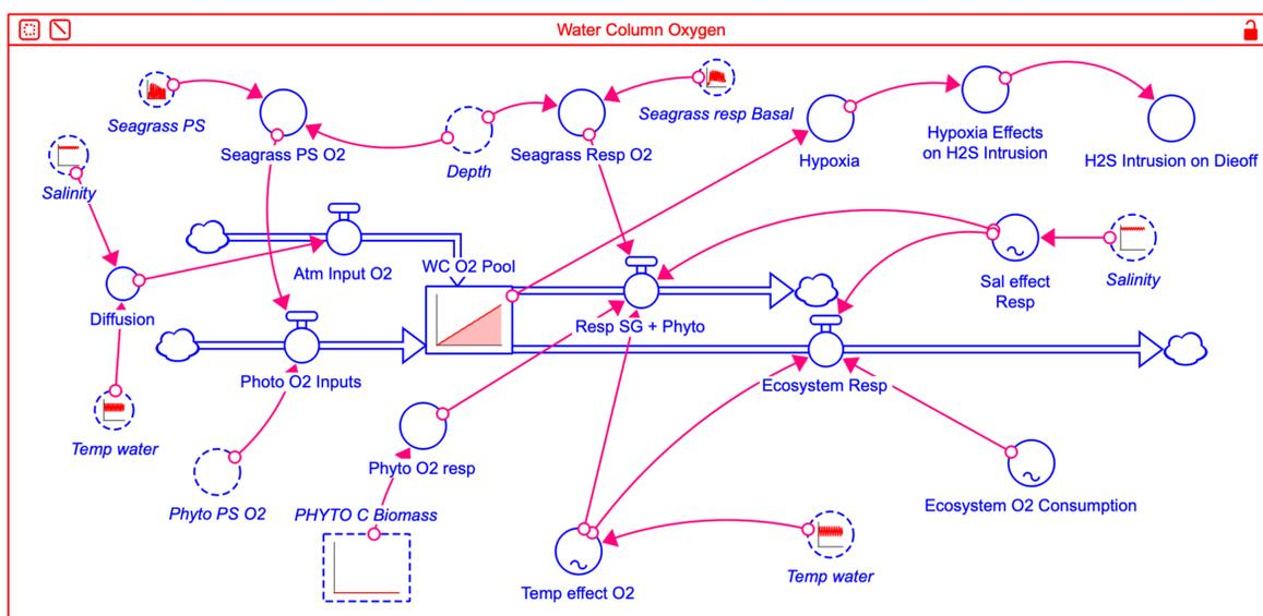
Figure 2: Water column oxygen module being developed to integrate into SEACOM. Oxygen inputs from seagrass, phytoplankton, and atmosphere are balanced by system respiration affected by temperature and salinity. Water column hypoxia effects are linked to seagrass sulfide intrusion, growth, and mortality (Stella Architect).
