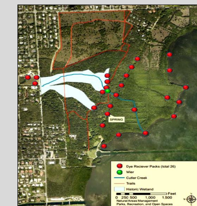
Dye test-determined where and how water is being distributed throughout Deering Estate Component
