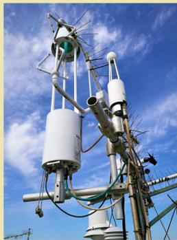
Eddy covariance (EC) is an approach to directly and continuously measure **net ecosystem CO<sub>2</sub> exchange (NEE)** between ecosystem and atmosphere.
