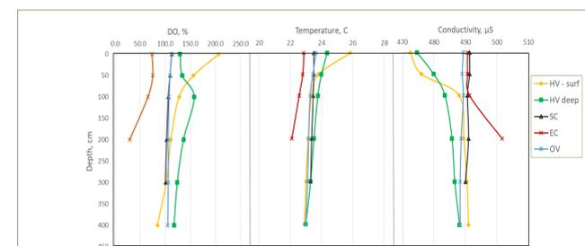
Fig. 8 Mean values of depth profiles of dissolved oxygen, water temperature and conductivity in stands of *Schoenoplectus* (SC), (*Hydrilla* (HV) and *Eichhornia* (EC) in July 2017 at San Lucas, Santa Catarina and San Pedro. HV – surf indicates values for a stand where the canopy is breaking water surface, HV – deep indicates stands with the canopy 50-150cm below the water surface.
