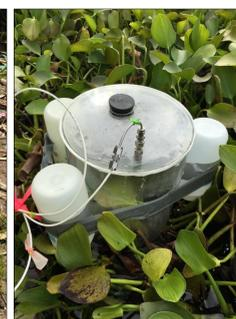
Fig. 5 The chamber for gas fluxes measurements
